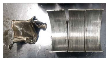
< Connecting rod bearing seizure >
