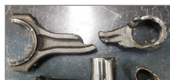
< Connecting rod broken >
